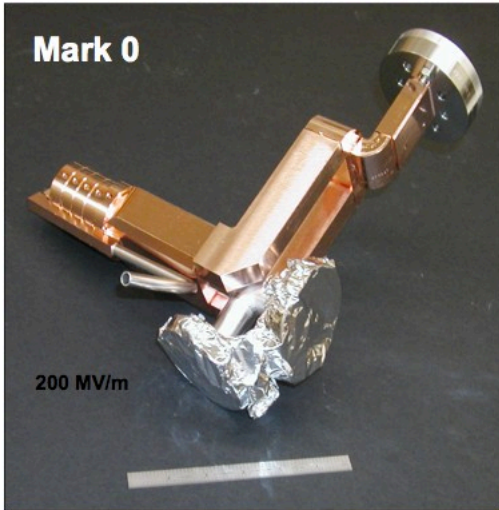
SLAC 5.5 cell x-band gun designed by Arnold Vlieks (SLAC)
